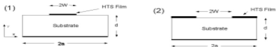
Fig. 1. The layout of microstrip line (1) and slotline (2) with superconducting strip
